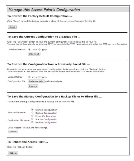
If you are experiencing problems with the UAP and have tried all other troubleshooting measures, click **Reset**. This restores factory defaults and clears all settings, including settings such as a new password or wireless settings. You can also use the reset button on the back panel to reset the system to the default configuration.
