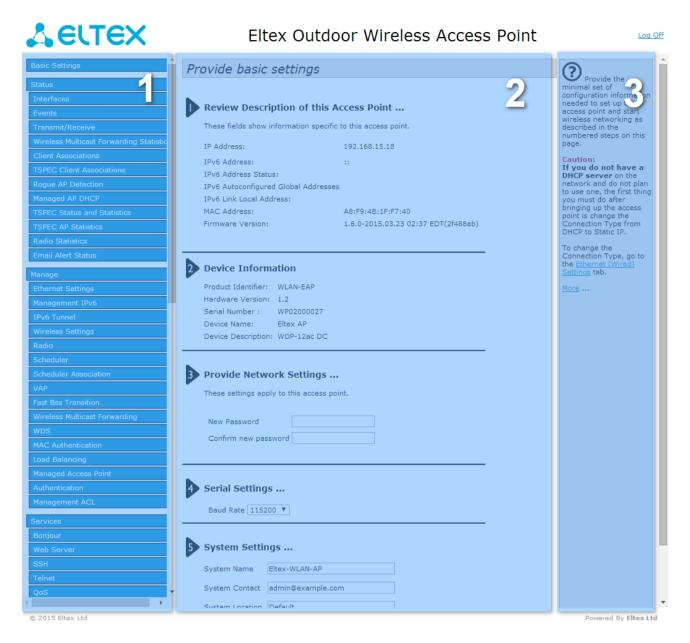
Fig. 1 – Web-confogurator navigation elements
