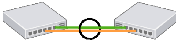
Fig. 16.1. Multiple Physical Links Combined to an Aggregation Group
