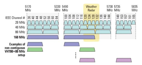
Channels used in a range of 5GHz when channel width is 20, 40 or 80 MHz
