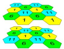
Scheme of channel allocation between neighboring access points that are located on different floors
