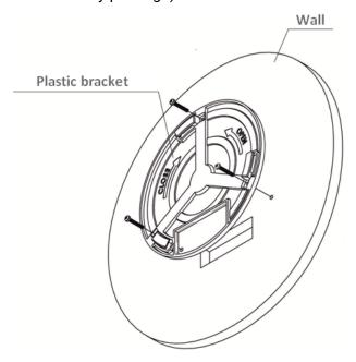
Attaching the bracket to a wall
